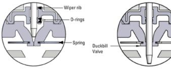
O-rings make sliding seal around needle
